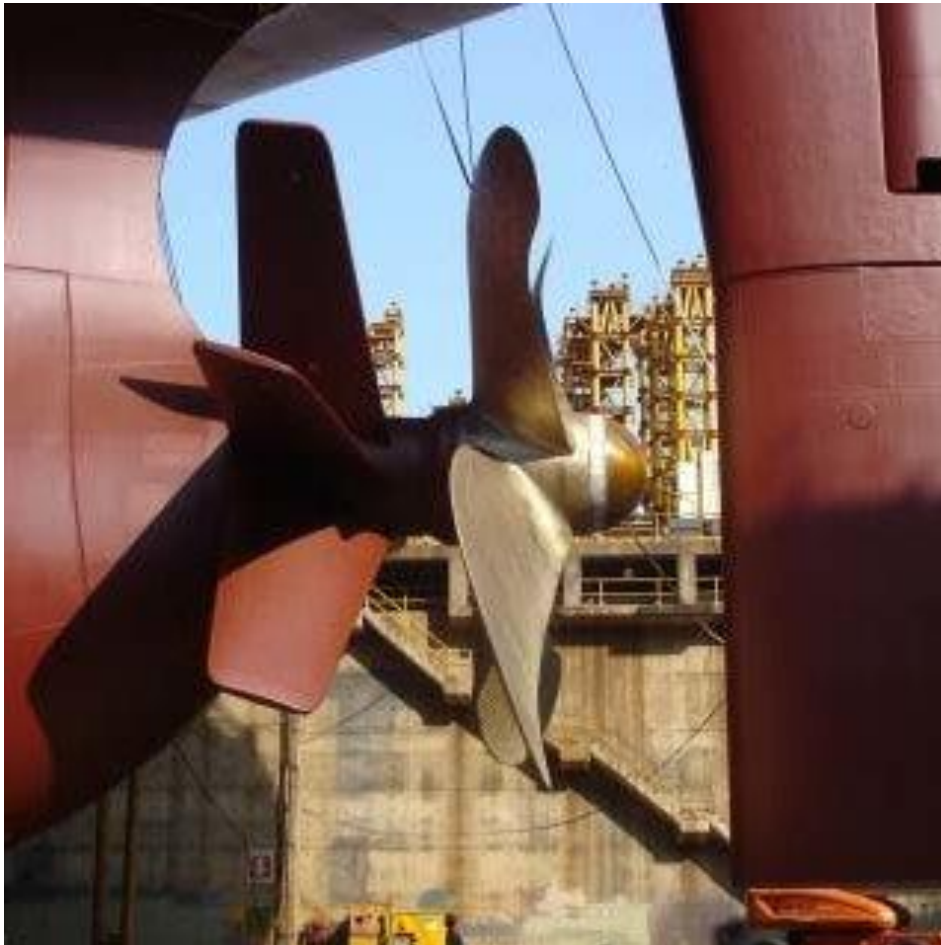
Sanoyas Tandem Fins. An Overview of Hydrodynamic Energy Efficiency Improvement Measures - Scientific Figure on ResearchGate. Available from: https://www.researchgate.net/figure/Sanoyas-Tandem-Similarly-to-the-aft-fin-of-the-Sanoyas-tandem-configuration-S
